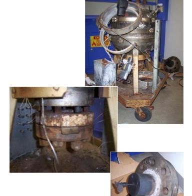
Most of the components attached to the vessel were rusted and therefore were removed. A Hydrotest was performed in order to verify equipment robustness at high pressures.
